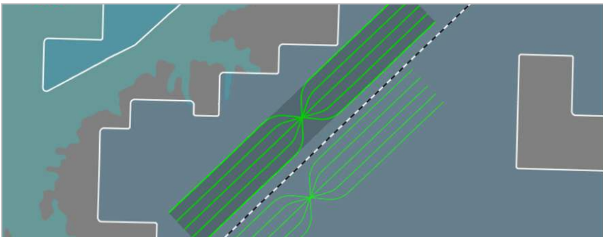
“Snap Align” feature automatically spaces your wells according to criteria that you specify
